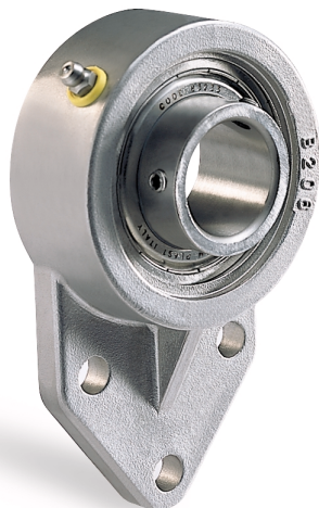
Flanged bearing in stainless steel series SS-UCFA for plain shafts d 20-25-30-35 mm
